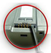
2. Taking care not to damage the cable, open the other side of the device by inserting the blade where shown below, then gently pushing up.
