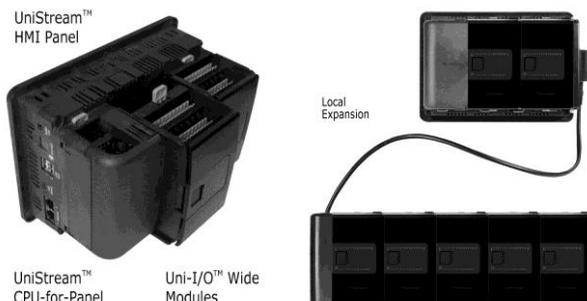
The maximum number of Uni-I/O™ Wide modules that can be connected to a single CPU controller is limited. For details, please refer to the specification sheets of the UniStream™ CPU or any of the relevant Local Expansion Kits.
