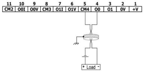
**Wiring the Analog Outputs**
