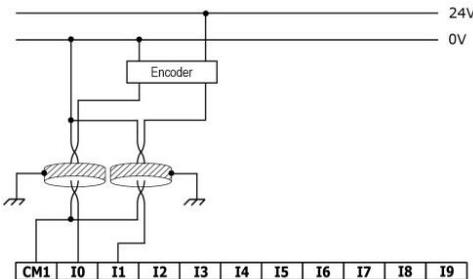
High Speed Input wiring, source
