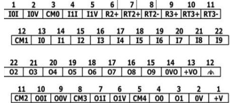
Wiring the Source Transistor Outputs
