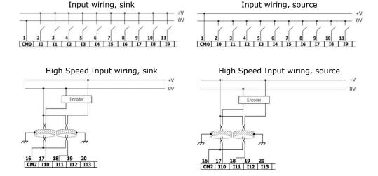
NOTE Use sink input wiring to connect a sourcing (pnp) device.
