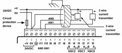
Analog input wiring, current (4-wire), voltage
