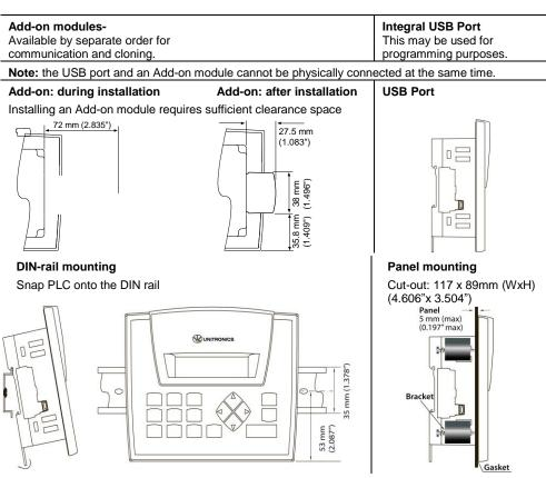
Note: Removing the unit requires clearance space. Recommendation: approximately 40mm (1.58"). For UL listed module, in order to meet the UL508 standard, panel-mount this device on the flat surface of a Type 1 enclosure.
