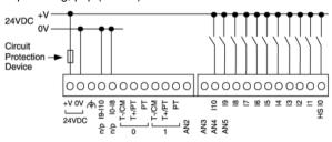
Input wiring, (I0-I8), pnp (source), (I9-I10), npn (sink)
