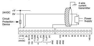
Analog Input wiring, voltage, AN4 and AN5
