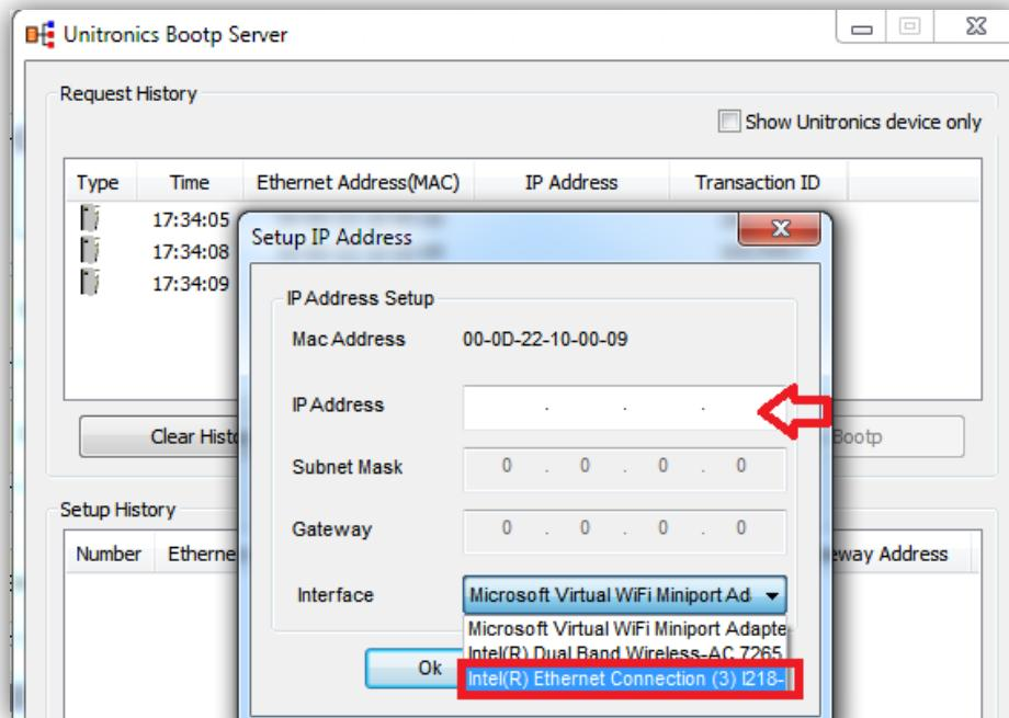
9. Click Ok. Now you should see the device in the bottom window including the IP address.
