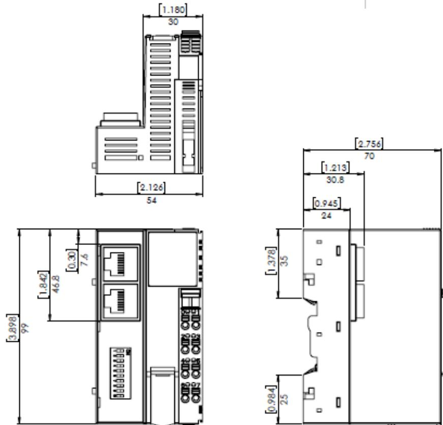
Installation - DIN-Rail Module Mounting
