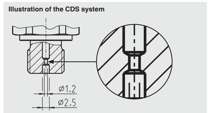
Fig. 1: Reduced diameter of the pressure channel
